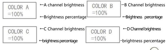
In this interface press plus / minus setting each channel brightness , press again  $\bigcirc$  can save exist setting , press  $\bigcirc$  for not save exist setting .
