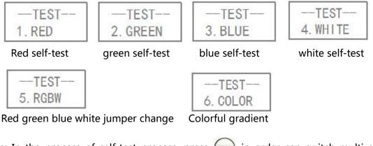
Note: In the process of self-test process ,press (rest) in order can switch multi self-test mode .
