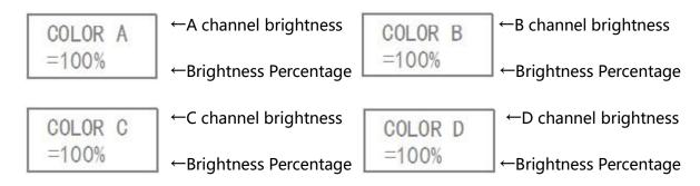
In the interface, press to set brightness, then press to exit with saving , press to exit without saving.
