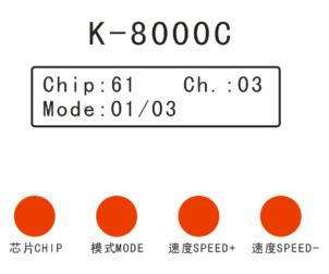
NOTE:61 means UCS512A or B coding mode; 62 means WS2821 coding mode; 63 means SM DMX512AP; 64 means UCS512-C; Ch.: 03 means the coding channel is 3 channels
